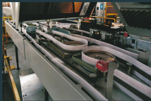
The sorting system automatically reads the field of the recipient and marks the letter with a bar code.
