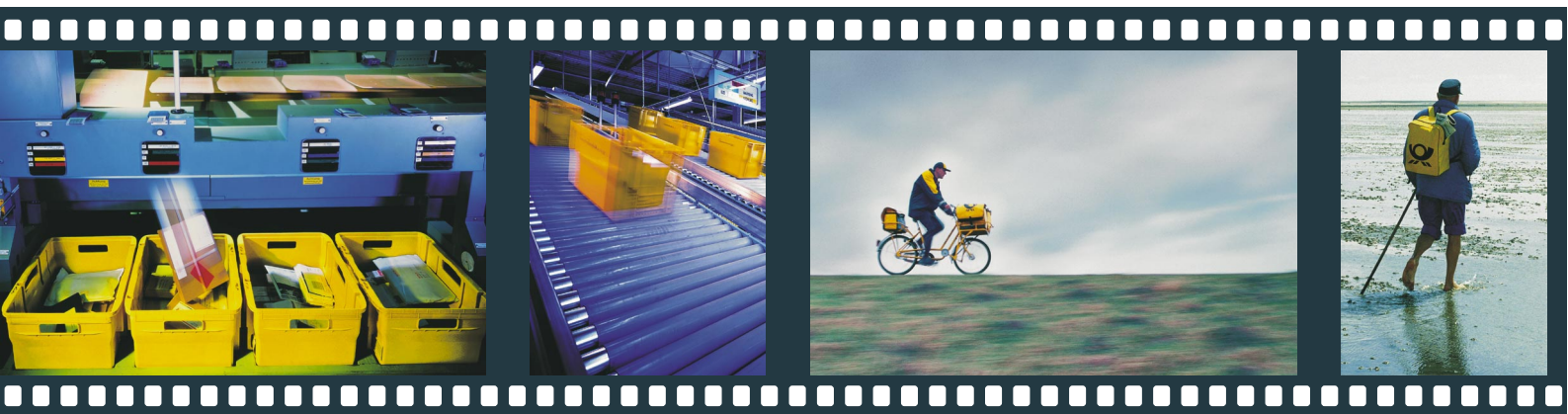
At the target letter center, the bar code is read and evaluated. A commissioning system sorts the letters for each mailman.
